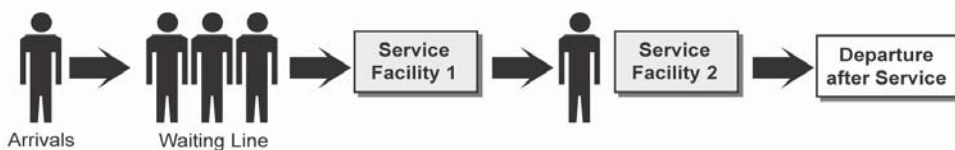
Figure 8.4: Single-channel, multi-phase system
